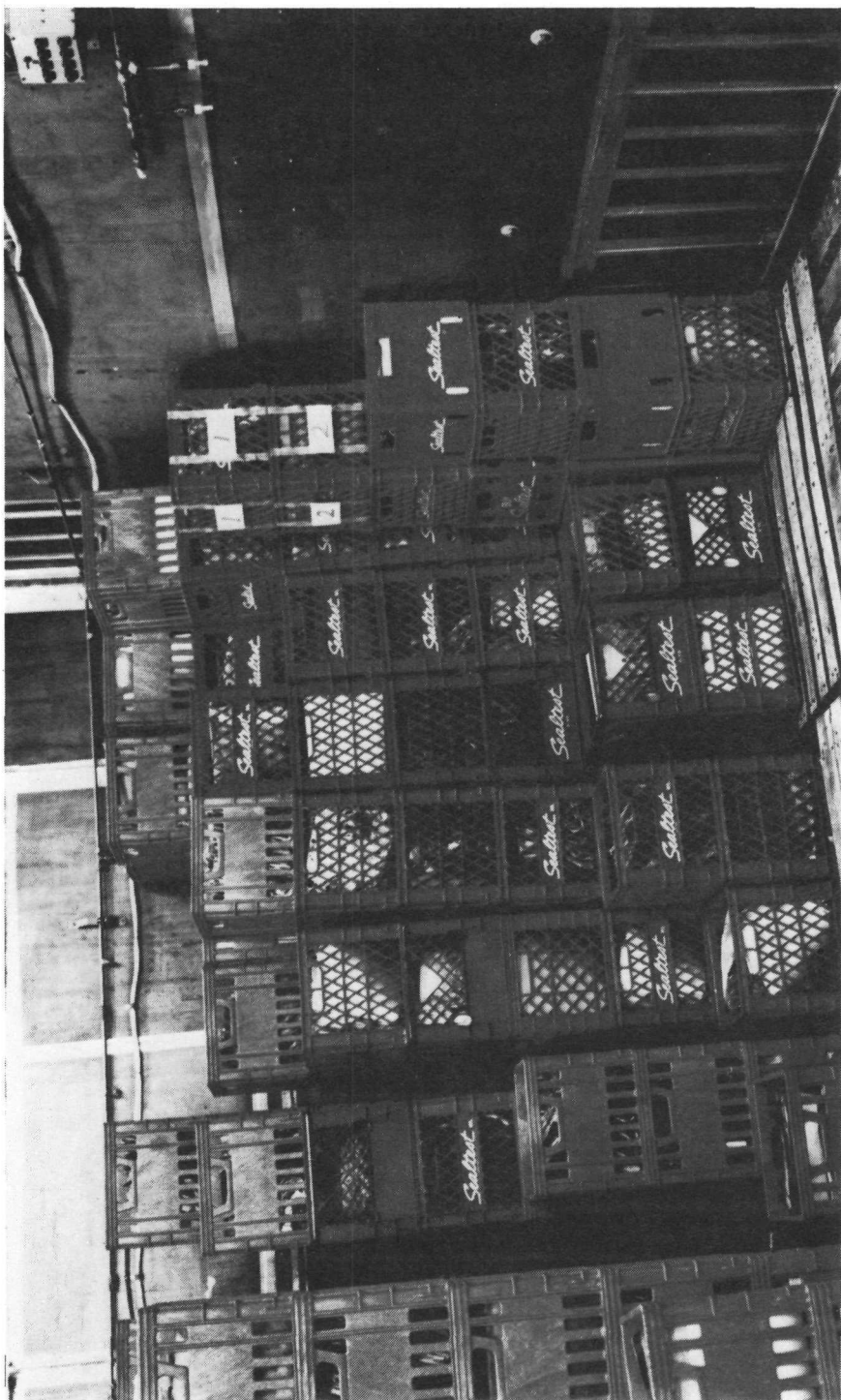
Records being vacuum dried in space simulation chamber at McDonnell Douglas Aircraft Corporation.
