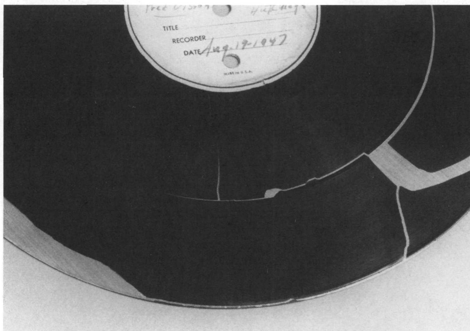
FIGURE 2. Aluminum-based instantaneous disc with shrinking, peeling coating.
