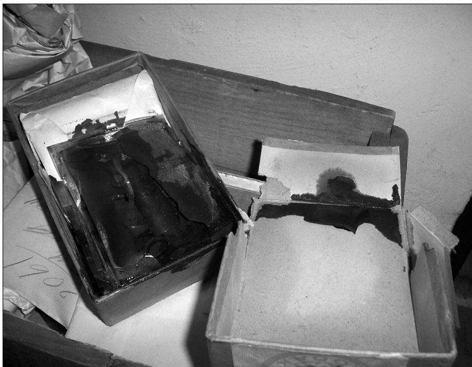
FIGURE 2. These are examples of embrittled film found in the collection.
