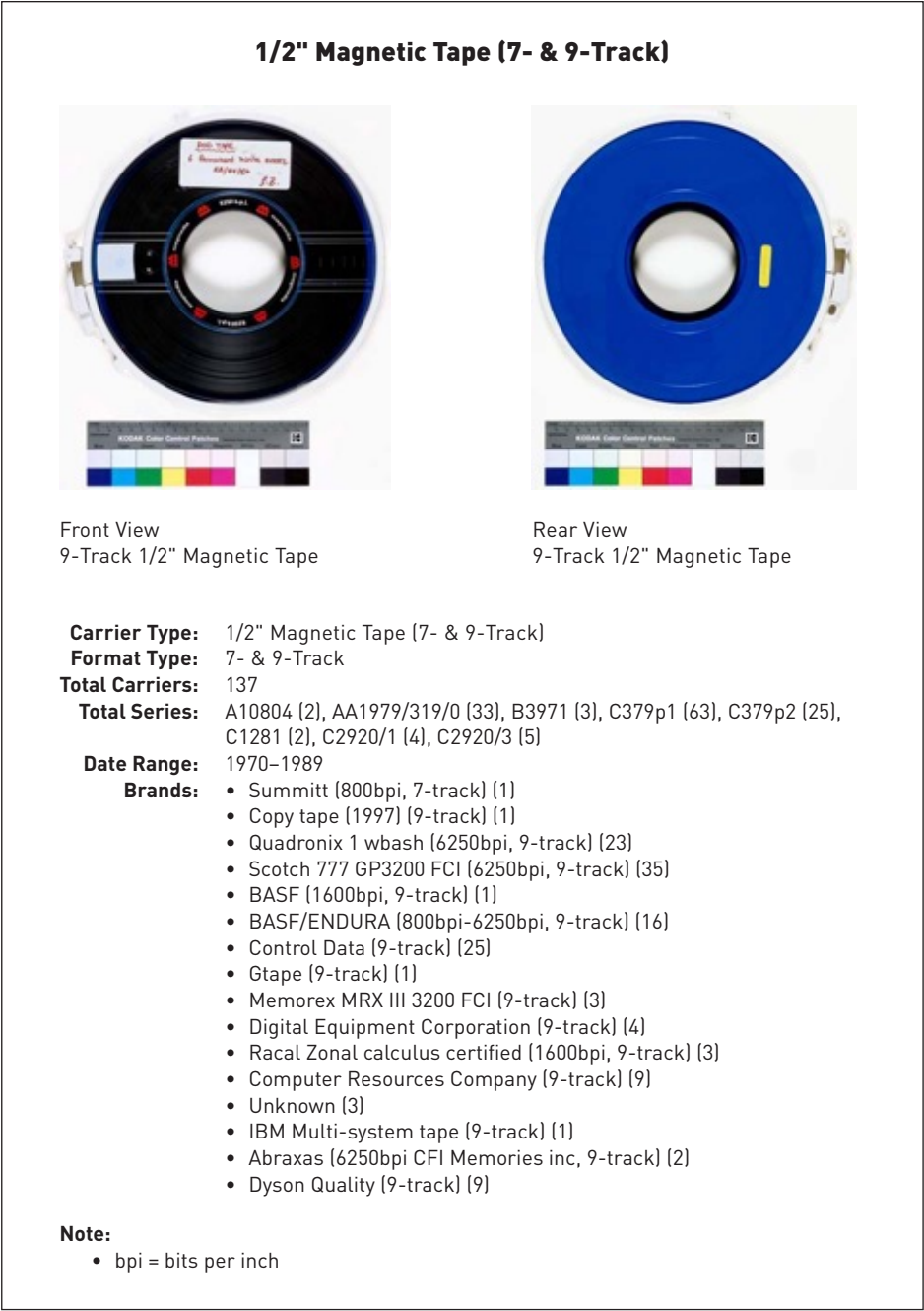
FIGURE 4. Details of 1/2" magnetic tape (7- and 9-Track) types used in the data recovery project (including brands, format density, etc.)
