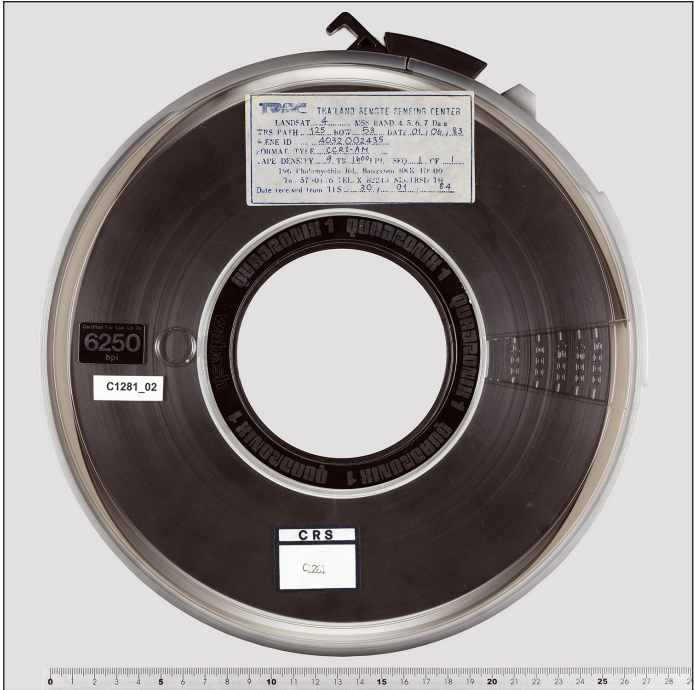
FIGURE 3. An image of the 9-track 1/2" magnetic tape that stored the original data (scale in cm). Descriptive metadata labels on the tape include the NAA accession numbers "C1281_2" and "CRS C1281"; information about the collection of the data on the tape (for details of the tape label, see Figure 4); and technical metadata about the manufacturer and the carrier type and capacity: "Wabash Quadronix 1" and "Certified For Use Up To 6250 bpi (bits per inch)." This type of information was collected and entered into the Carrier Treatment Check Sheets.
